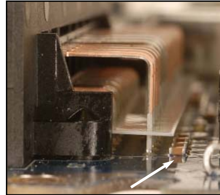
Figure 2. Filter capacitor very near to thru-hole connector.
